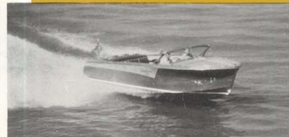
Model 120 and Model 120-S - 24 ft. sedan or utility with twin power up to 225 H.P. - vee drive installation - wooden framed windshield - two extra seats or liquor cabinet and ice box optional.
