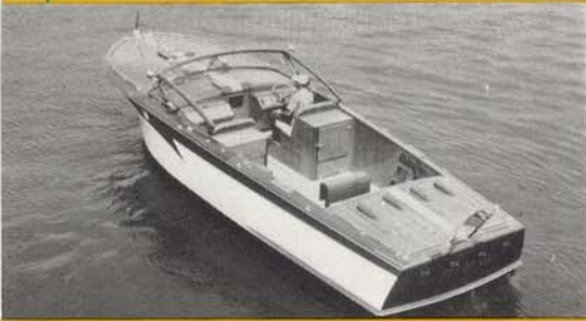
Model 155A - 30 ft. commuter with convertible top standard equipment - power to twin 225 H.P. vee-drive - designed for all day offshore trips. Sleep two.
