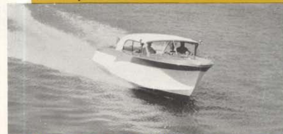
Model 130 and 150 - 27 ft. utility or sedan accommodation - power up to 275 H.P. - vee-drive installation - ice box, hand basin, liquor cabinet, sleeping accommodation for two, forward.
